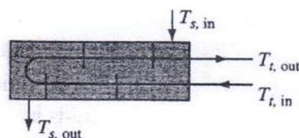
Correction factor to counterflow LMTD for heat exchanger with one shell pass and two (or a multiple of two) tube passes.
