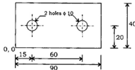
The drill rotates at 500 rpm and feed rate is 200 mm/min. How do you code the information in—
