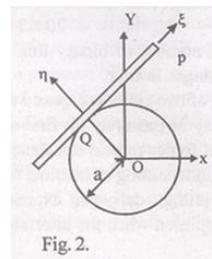
**(b)** A rigid rod (Fig. 2) slides over a fixed circle of radius  $a$ . The distance of rod's tip  $P$ , measured from the contact point  $Q$  is denoted by  $s$ , and the rod makes an angle  $\phi$  with the fixed  $x$ -axis. Find the acceleration components  $(a_x, a_y)$  of point  $P$  with respect to the fixed frame  $(X, Y)$ , also find the components  $(a_\xi, a_\eta)$  of the absolute acceleration in the direction of moving axes  $(\xi, \eta)$ . 20
