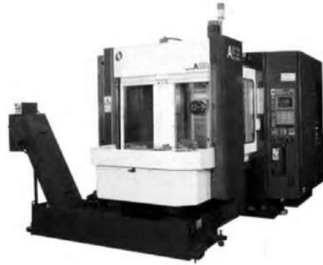
Fig. 9.12 Present-day production horizontal axis CNC machining centre Makino A55 (Courtesy, Makino Milling Machines Co. Ltd., Tokyo, Japan)
