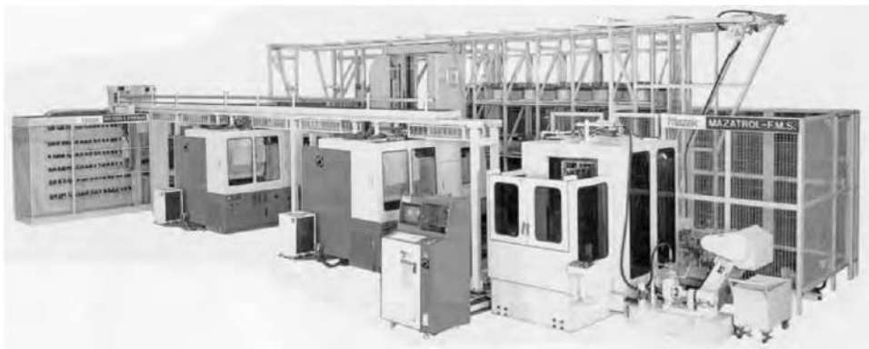
Fig. 22.10 Tool hive integrated with a FMS using tool transfer robot moving on the monorail. (Courtesy, Yamazaki Mazak Corp., Japan)
