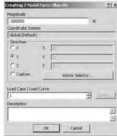
Fig. 8.26 Specifying the acting force in Algor
