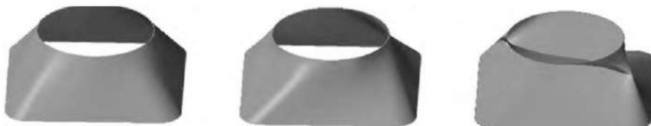
Fig. 4.22 Different ruled surfaces obtained from the same closed curves. The different surfaces resulted because of the differences in the selection of the starting point on each of the curves
