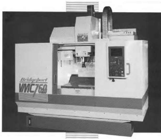
Fig. 12.1 Present-day production vertical axis CNC machining centre Bridgeport VMC 760 (Courtesy, Bridgeport Machines Inc., Bridgeport, USA)
