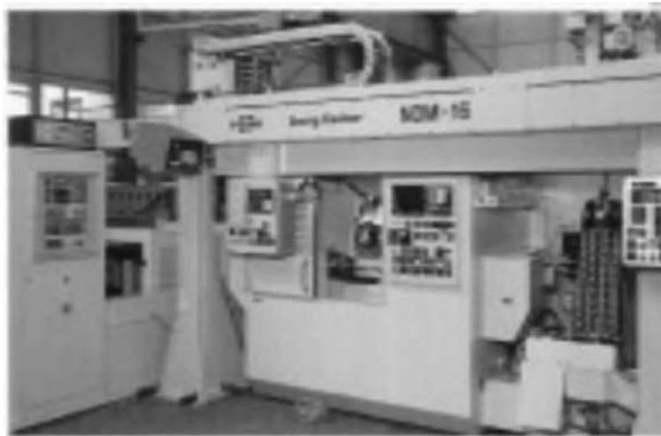
Fig. 11.23 Drum-type tool magazine used in CNC turning centres with modular tooling for storing large number of tools (Courtesy, Georg Fischer, Switzerland)
