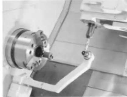
Fig. 11.13 Typical tool setter integrated with a CNC turning centre (Courtesy, Yamazaki, Japan)
