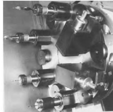
Fig. 12.20 A tool turret with driven tooling to be used in a CNC turnmill centre (Courtesy, George Fischer, Switzerland)
