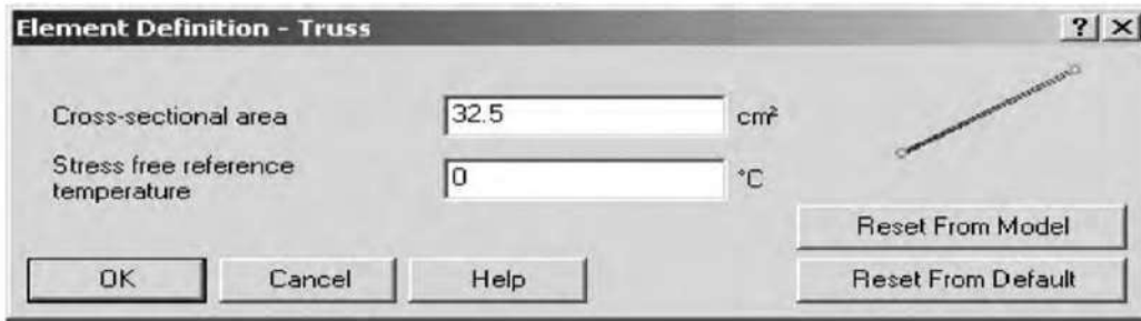
Fig. 8.23 Specifying the geometric properties of the truss element in Algor
