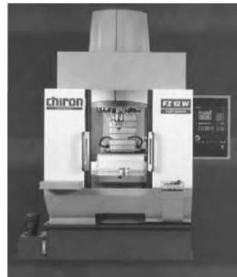
Fig. 12.8 Chiron CNC machining centre FZ 12W for high-speed machining with a very fast tool-change time (Courtesy, Chiron Werke GmbH, Germany)
