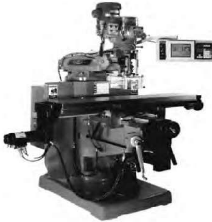
Fig. 9.11 Early form of CNC milling machines: EZ-TRAK DX II milling machine (Courtesy, Bridgeport Machines Inc., Bridgeport, USA)
